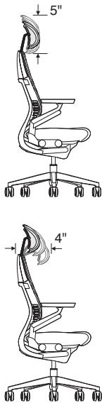
Headrest adjusts 5" vertically and measures 8"H x 10 $\frac{1}{2}$ "W. It tilts 4" forward and the cushion rotates 90°. Plastic shell on the headrest is available in black, merle, or seagull and will match the plastic back shell. Upholstery can match or contrast the seat and back material. It is not available to order separately for installation on existing Gesture chairs. Headrest is available on stools as a special only.
