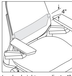
Lumbar height adjusts 4" (5 1/4" to 9 1/4") from seat by grabbing exposed tabs and sliding the lumbar support up or down. This feature is optional on work chairs and stools.
