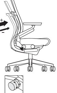
Back tension. Turn the knob forward for more resistance and backward for less resistance. Adjust back tension for appropriate amount of resistance.
