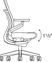
Passive seat edge angle flexes 1 1/2", relieving pressure under the user's thighs. This feature is standard on all work chairs and stools.
