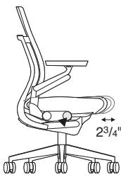
Seat depth adjusts 2 3/4" (15 3/4" to 18 1/2") by rotating dial while seated for an easy fine-tuned fit. This feature is standard on work chairs and stools.
