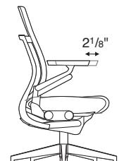
Arm depth adjusts 2 1/8" to enable user to get closer to worksurface.
