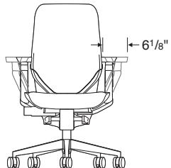
Arm width adjusts parallel 6 1/8" per arm for a total range of 10 1/4" to 22 1/2" between arms.
