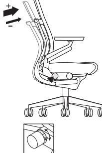
Variable back stop. To lock backrest in upright position, lean forward and flip lever down. Flip lever up to unlock for full-range motion. There are four settings to give just the right angle of recline.
