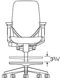
Column and foot ring on stools adjusts by first lifting ring and rotating it counterclockwise to unlock. Then raise or lower ring up to 3 3/4" to desired position before rotating it clockwise to lock.
