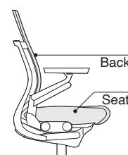
Seat and back cushions can be removed and replaced if damaged.
