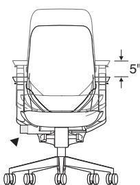
Seat height adjusts pneumatically. To lower, hold handle up while seated. To raise, hold handle up and keep weight off the chair. Range of adjustability is 5", from 16"H to 21"H, and is standard on work chairs. An optional 5 1/2" high-range of adjustability (17 1/2"H to 22 1/2"H) and a 3 3/4" low-range (14 1/2"H to 18 1/4"H) are available as an option. Stools are standard with an 8 1/4" range of adjustability (24"H to 32 1/4"H).
